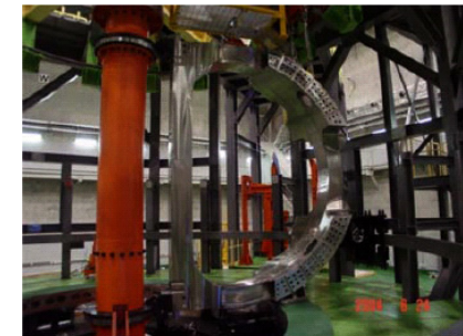
Fig. 9 The TF00 magnet after assembly test
