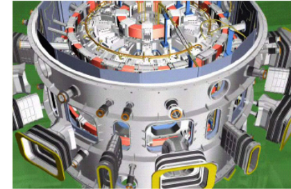
Fig. 4 Schematic drawing - assembling the vacuum vessel ports
