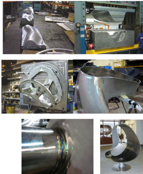
1. Fabrication of the NCSX Prototype Vacuum Vessel Segment
